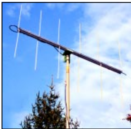
The LPDA with elements oriented vertically. Use this orientation only with a nonconductive mast.
