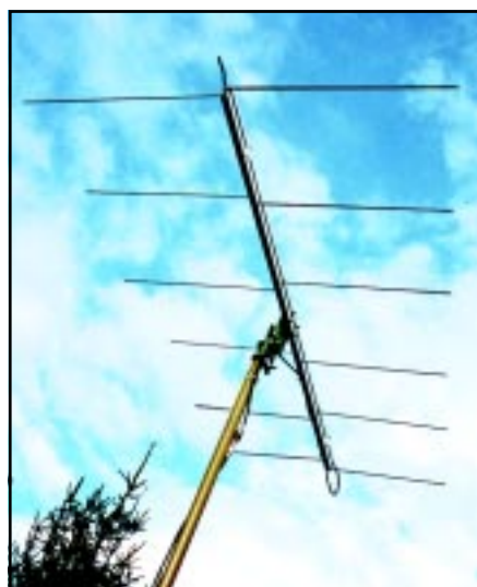
The LPDA with elements oriented horizontally.
