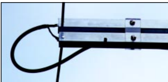
View of the front of the LPDA showing the elements, the feed-line mounting system and the front Plexiglas boom insulators.
