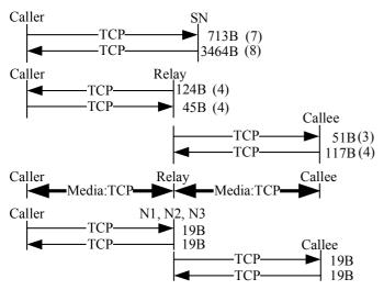
Caller and callee on the average exchange 3 msg/s over TCP with N1, N2 and N3 after call has been established.
