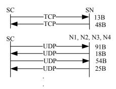
Figure 6. Message flow for a successful user search when SC v1.4 is behind a port-restricted NAT. 'B' stands for bytes and 'N' stands for node. UDP packets were sent to N1, N2, N3, and N4 during login process and responses were received from them. Message size corresponds to payload size of TCP or UDP packets. Not all messages are shown.
