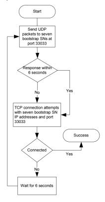
Figure 3. Skype login process. SC sends UDP packets of length 18 bytes to all bootstrap SNs. After 5s, it attempts TCP connections with the seven bootstrap SN IP address and ports 33033. Authentication with the login server is not shown.
