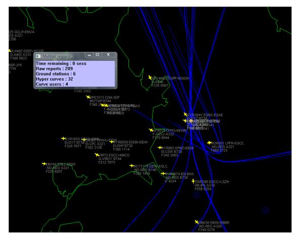
The overall requirement for successful multilateration is for data bursts from the wanted aircraft, together with data bursts from suitable reference aircraft (ones that report position), to be received by at least three well-distributed Ground Stations. This, together with some critical timing constraints, explain why positive results are by no means guaranteed.
